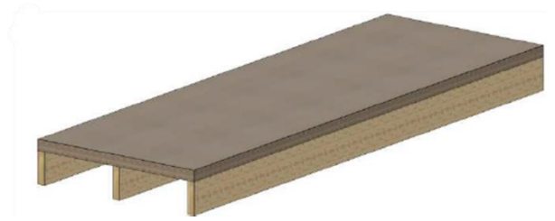
Figure 1-2: Open box with outer webs flush with flange
