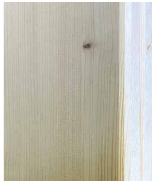
CLT element, special surface spruce
